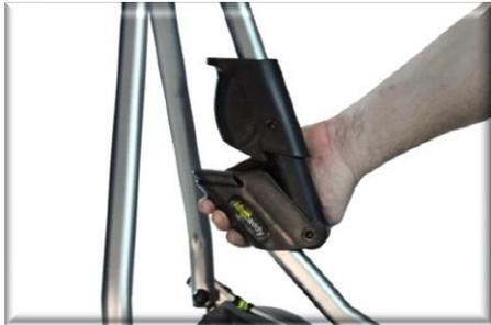
Slide the lower frame folding lock as shown and lift the handle to release the rest of the frame.
