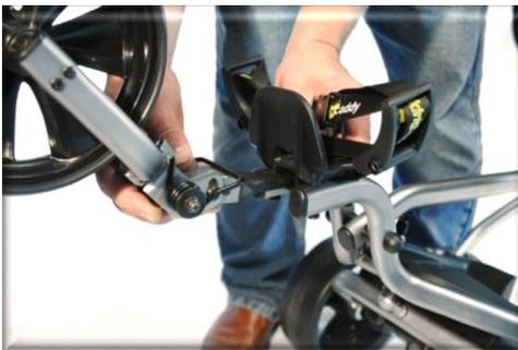
Locate the front wheel assembly and align the assembly with the main frame as shown.
